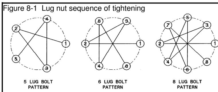
Keep a record of the date and approximate mileage when you check the lug nut torque. Note any lug nut that has lost torque. Investigate the reason(s) if the lug nut torque is not maintained after more than one re-torque application, because this indicates there is something wrong with the lug nuts, nut studs, wheels and/or hubs and should be corrected.
